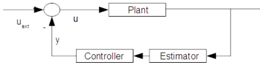
**Fig 1 Single-loop feedback**
