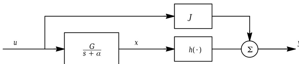
**Figure 1** A nonlinear system with linear dynamics
